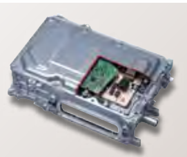
DC-DC converter mounted in the new Prius
